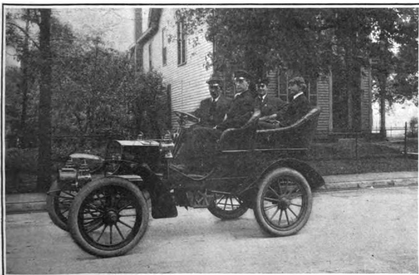
The photograph herewith reproduced shows the new four-cylinder air-cooled Premier tonneau car built by the Premier Motor Manufacturing Company, of Indianapolis. The occupants are: Front seat, H. O. Smith, president, and at the wheel, George Weidley, superintendent of the shops; rear seat, front view, Carl Fisher; side view, Lucian M. Wainwright.
